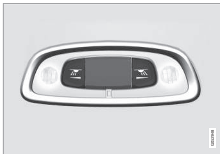
Reading lamps above the second 26 and third seat row*.
