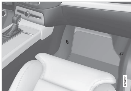
Mounting point locations in the front seat.
