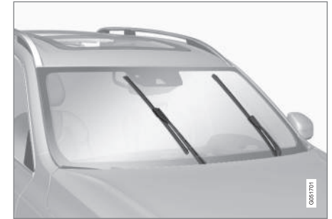
Wiper blades in service position.
