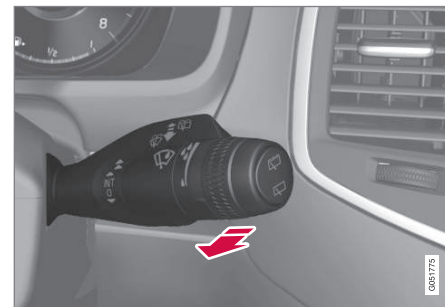
Washing function, right-hand stalk switch.
