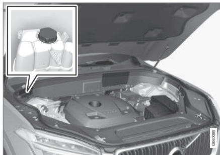
Coolant expansion tank.
