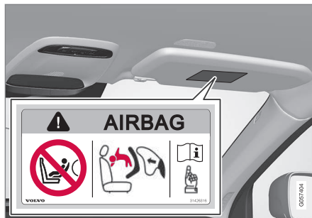
Label on the passenger side's sun visor.
