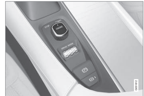
Start knob in the tunnel console.
