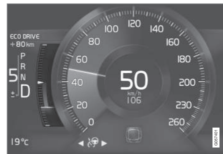
Eco gauge in the 8-inch driver display.
