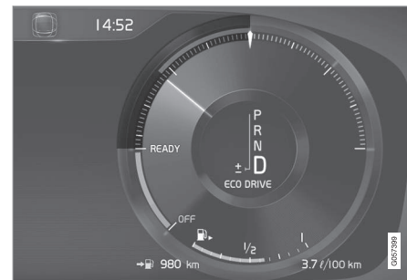
Eco gauge in the 12-inch driver display.
