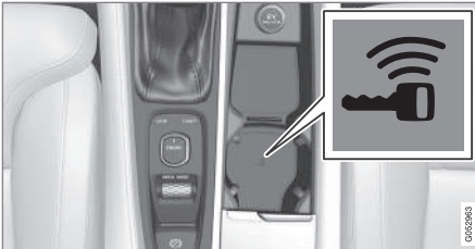
Back-up reader in the tunnel console
