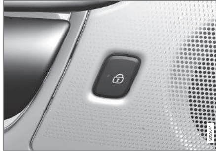
Rear door lock button and indicator light
