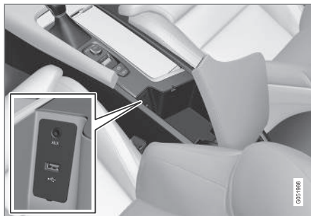
USB socket in the tunnel console
