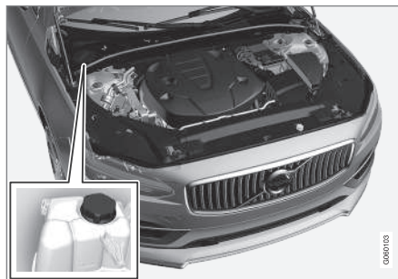
Coolant expansion tank
