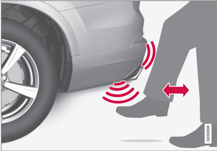
Kicking motion under the sensor's activation area
