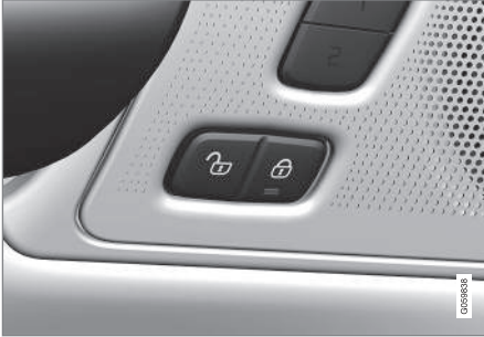
Front door lock button and indicator light
