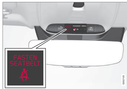
Seat belt reminder light in ceiling console
