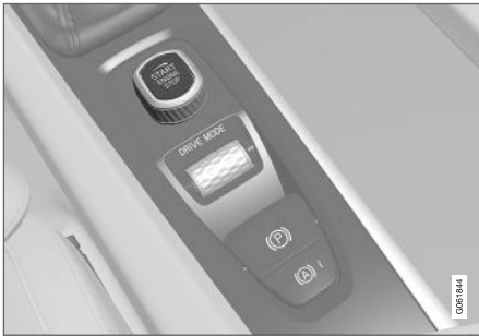
Start knob in the tunnel console.
