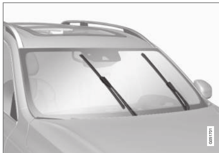
Wiper blades in service position.
