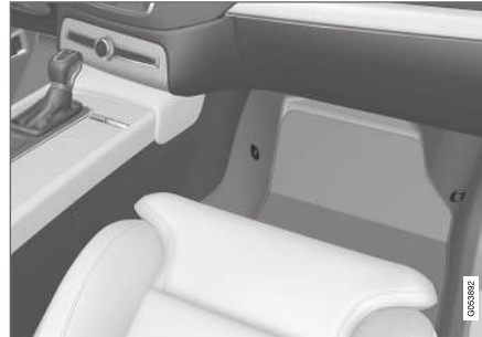
Mounting point locations in the front seat.
