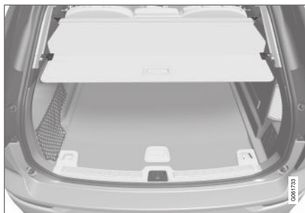
Cargo cover in full-cover position.
