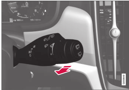
Washing function, right-hand stalk switch.
