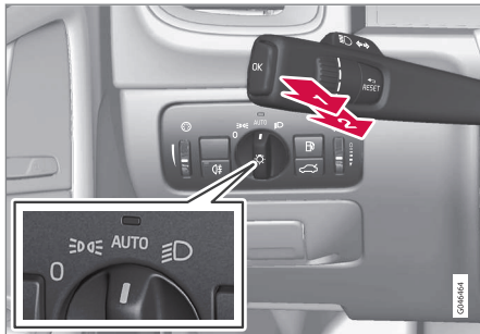
Stalk switch and knob for headlamp control.
