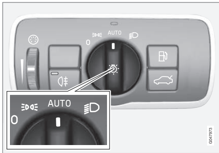
Knob for headlamp control in AUTO position.
