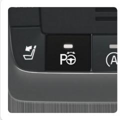
PAP checks the available space, and then steers in the car. Your task is to select the gear, control the speed and brake/stop.
