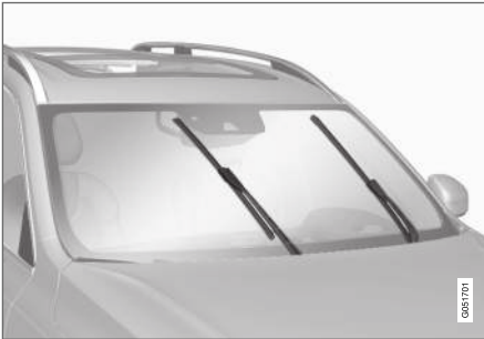
Viskerblader i servicestilling.
