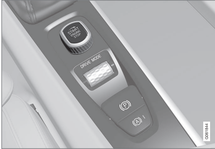
Start knob in the tunnel console.
