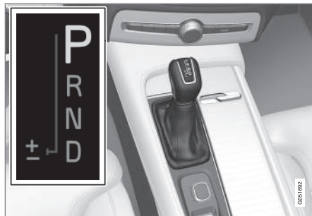
Overview of large gear lever and shift pattern in the driver display.
