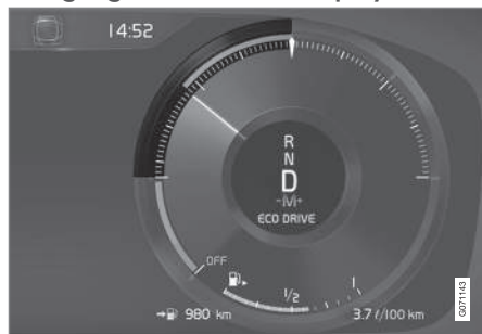
Eco gauge in the 12-inch driver display*.
