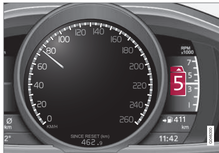
Combined instrument panel "Digital" with gear shift indicator.
