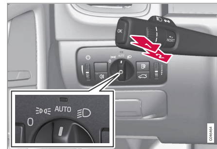
Stalk switch and knob for headlamp control.
