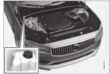
Coolant expansion tank, left-hand drive vehicle.
