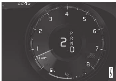
Instrument panel when the paddles are activated for shifting.
