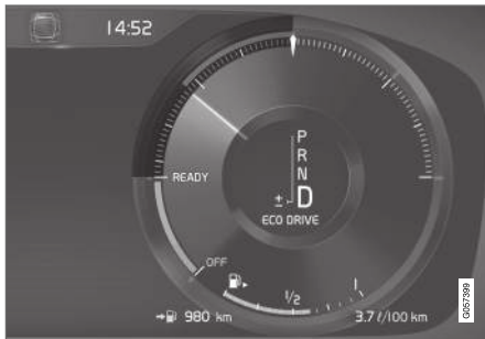
Eco gauge in 12" instrument panel*.
