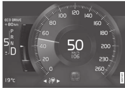
Eco gauge in 8" instrument panel.
