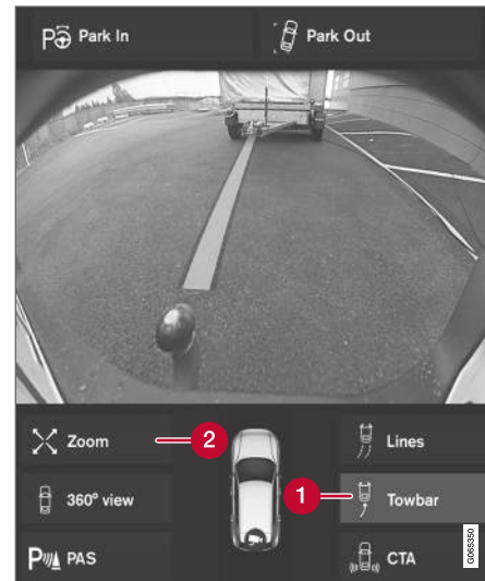
Towbar with trajectory line.
