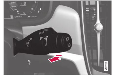
Washing function, right-hand steering wheel lever.
