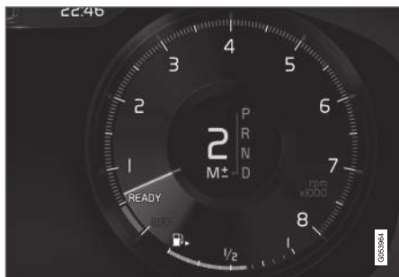
Instrument panel when the paddles are activated for shifting in manual mode.
