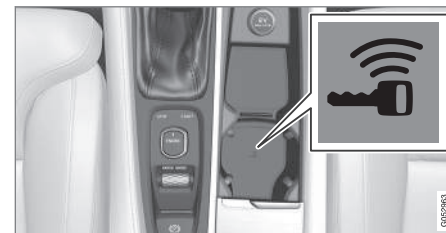
Backup reader's location in the tunnel console.
