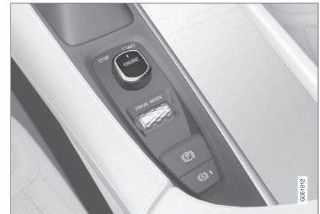
Start knob in the tunnel console.
