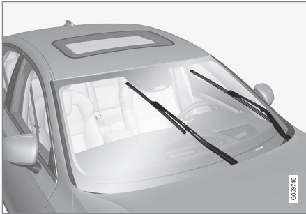
Wiper blades in service position.
