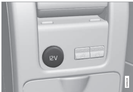
12 V socket in tunnel console, rear seat.
