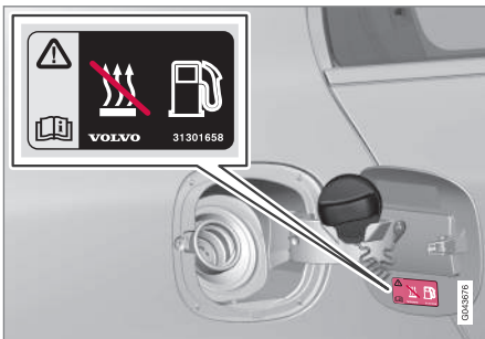
Warning label on fuel filler flap.
