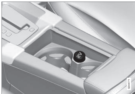
12 V socket in tunnel console, front seat.
