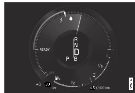
The driver display for propulsion with both the electric motor and internal combustion engine.
