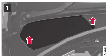
Coolant expansion tank, right-hand drive car.
