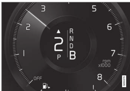
Gear shift indicator in the driver display 5 .
