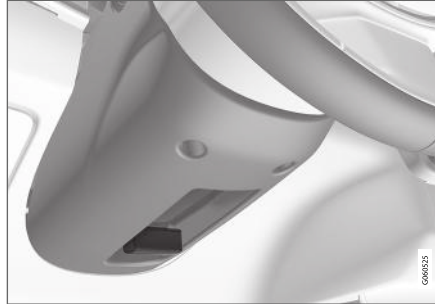
Lever for steering wheel adjustment.
