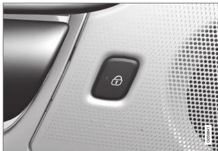
Locking button with indicator lamp in the rear door.
