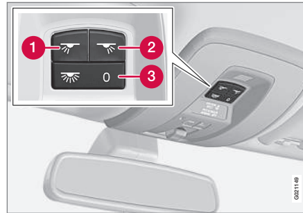
Light switches, front roof lighting
