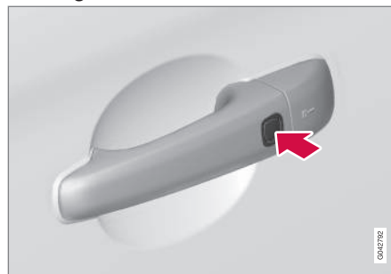
Models with keyless drive have a button on the outside door handles
