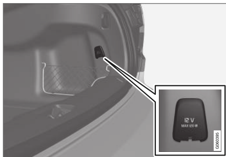
12 V electrical socket in cargo area*.
