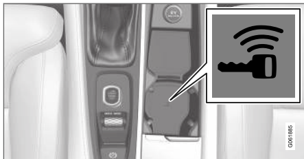
Backup reader's location in the tunnel console.
