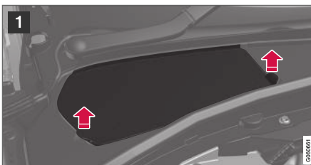
Coolant expansion tank, right-hand drive car.
