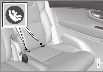
Location of the ISOFIX/LATCH anchors
