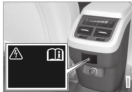
Electrical outlet in the tunnel console, second row of seats.
