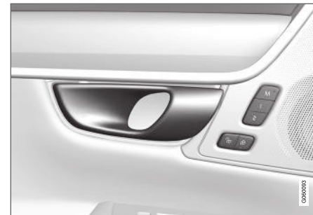
Opening handle for alternative unlocking in the side door 12 .
