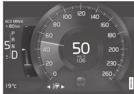
Eco gauge in the 8-inch driver display.
