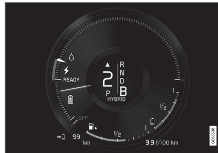
The driver display indicates charging during engine braking.
