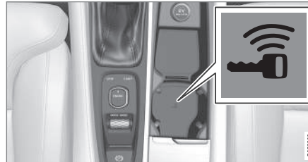
The backup reader's location in the tunnel console.
