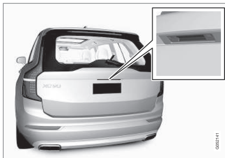
Rubberised pressure plate on the tailgate used for unlocking only.
