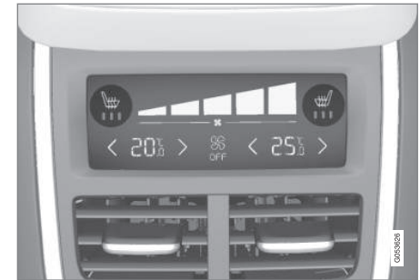
Seat heating indication and controls on the climate panel at the rear of the tunnel console.
