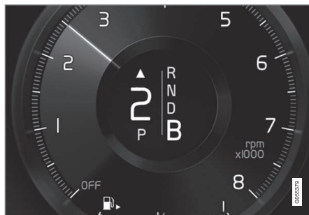
Gear shift indicator in the driver display 2 .
