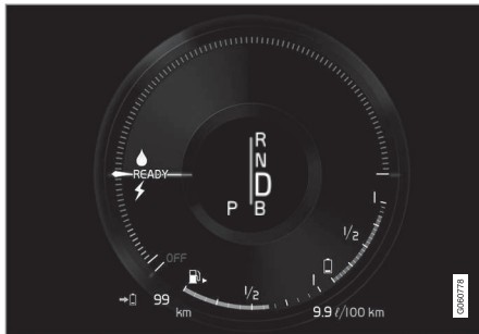
The car is started but stationary, no power is requested.
