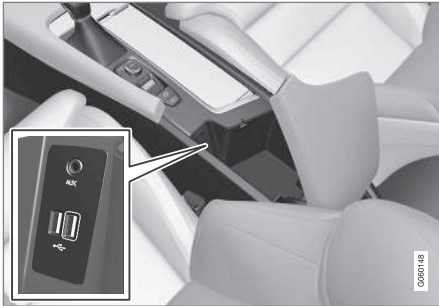
USB socket in tunnel console.
