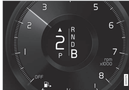
Gear shift indicator in the driver display 2 .
