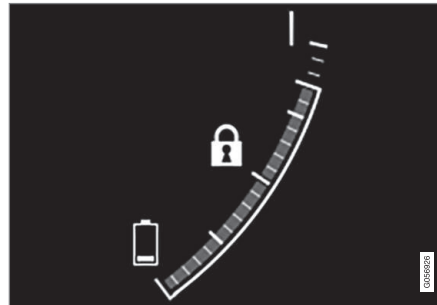
The car generates current to the battery, the battery is charged, e.g. when the brake pedal is pressed lightly or during engine braking down a hill.
