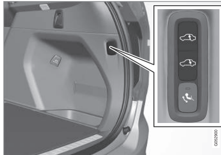
Controls for raising/lowering the car's rear section.
