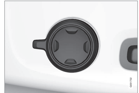
Multi-function control, located on the side of the seat's seating section.
