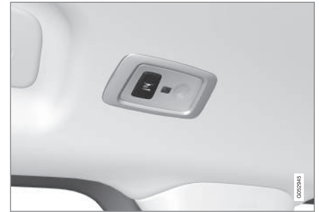
Reading lamp above the second seat row in cars with panorama roof*.
