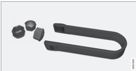
Tool for removing the plastic caps on the wheel bolts.
