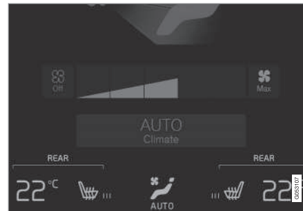
Buttons for heated seats in the group Rear climate in the climate view.
