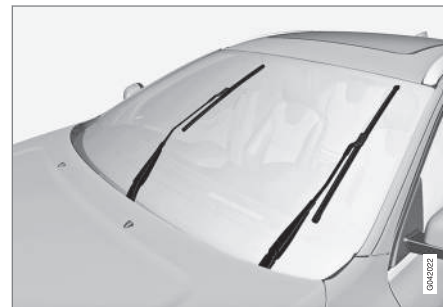
Viskerblade i servicestilling.
