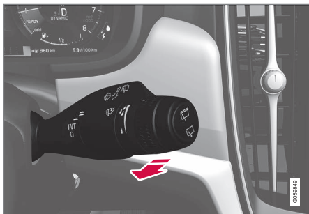
Washing function, right-hand steering wheel lever.
