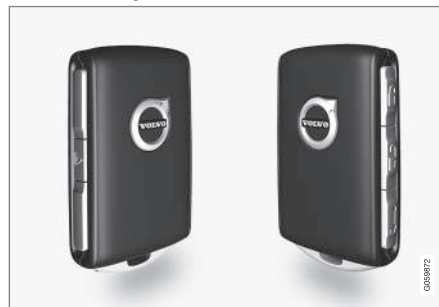
The remote key has four buttons, one on the left side and three on the right.
