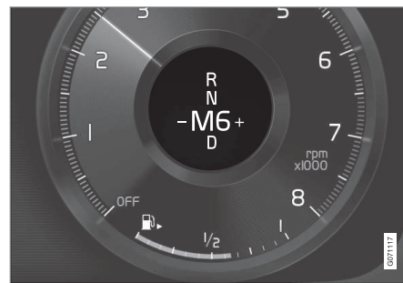
Overview of gear shift pattern in the instrument panel for small gear selector.
