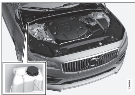
Coolant expansion tank, left-hand drive vehicle.
