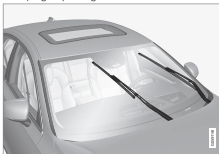
Windshield wipers in the service position.
