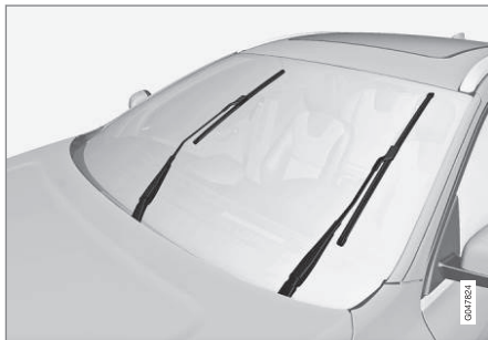
Viskerblade i servicestilling.
