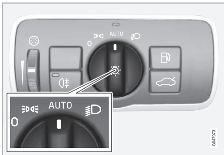
Headlight switch in the AUTO position
