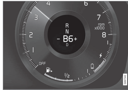
Gear shift indicator in the driver display 5 .
