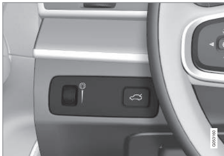
Thumbwheel (to left) for adjusting interior brightness.
