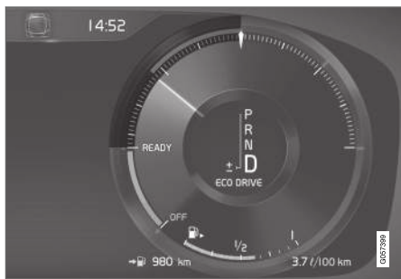
Eco gauge in the 12-inch driver display*.
