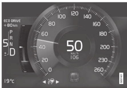
Eco gauge in the 8-inch driver display.
