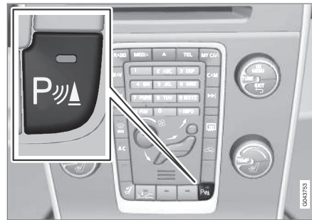
On/Off for parking assistance and CTA sensors.
