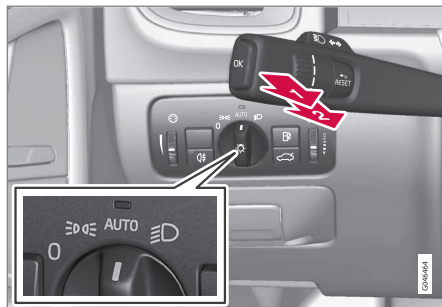
Stalk switch and knob for headlamp control.
