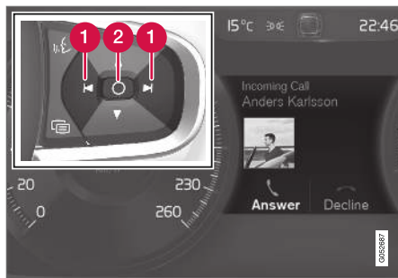
Examples of messages in the instrument panel 7 and the right-side steering wheel keypad.
