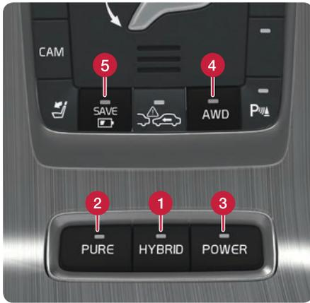
The car is powered by two motors - an electric motor and a diesel engine. Different drive modes can be selected. It is not possible to select the "wrong" drive mode - the car returns to the HYBRID mode if certain conditions are not met. The lamp in the hybrid button will then illuminate.
