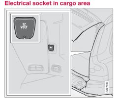
Slide down the cover when you wish to use the socket. It works regardless of whether the ignition is on or off.
