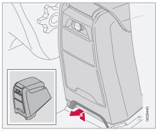
The centre console must first be removed if you wish to slide the centre seat in the second row forward.
