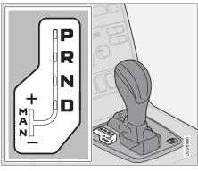
To move from the automatic driving position  ${\bf D}$  to a manual position, move the gear selector to position  ${\bf M}$ . To go from position  ${\bf M}$  to the automatic driving position  ${\bf D}$ , move the selector to position  ${\bf D}$ .
