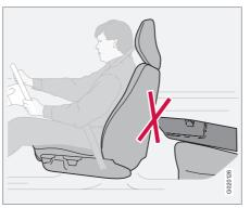
Do not place objects in the rear seat that may prevent the WHIPS system from functioning.
