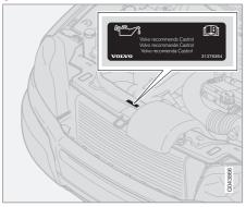
Using oil of a higher than specified grade is permitted. If the car is driven in adverse conditions, Volvo recommends using an oil of a higher grade than that specified on the decal, see page 277.
