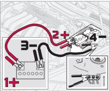
If the battery in the car has become discharged, you can "borrow" electric current from either a separate battery or from another car. Always make sure the crocodile clips on the jump leads are attached securely to eliminate sparks during the start attempt.
