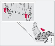
The passenger seat backrest can be folded forward to make room for long loads.
