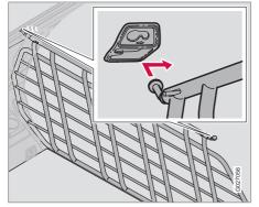
The protective grille in the cargo area prevents cargo or pets from being thrown forward in the passenger compartment in the event of heavy braking.
