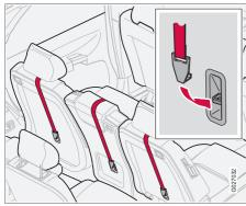
The car is equipped with upper mounting points for child seats. These mounting points are located on the rear of the rear seats.
