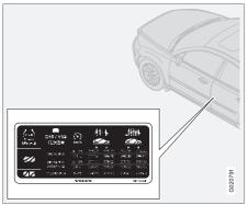
The tyre pressure label on the driver's side door pillar shows which pressures the tyres should have at different loads and speed conditions. Stated on the decal:
