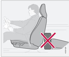
Do not leave any objects on the floor behind the driver's seat/passenger seat that may prevent the WHIPS system from functioning.
