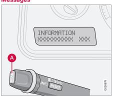
When a warning or indicator symbol illuminates, it is supplemented by a message appearing on the display.
