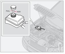
**i** NOTE Check the level frequently. Check the level frequently. The fluid does not require changing. The level must lie between the **ADD** and **FULL** marks. See the capacities and recommended grade on page 279.
