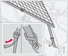
If the car is equipped with a cargo area cover, remove it before fitting the safety net.
