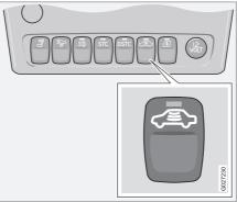
If someone is going to stay in the car but the doors must be locked from the outside, then the deadlocks function can be temporarily switched off.
