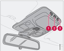
Controls in roof console for front reading lamps and passenger compartment lighting.
