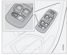
All the doors and the tailgate can be locked or unlocked simultaneously using the control panel in the driver's door (or passenger door).
