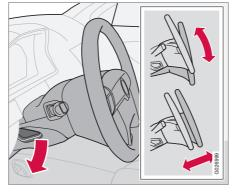
The steering wheel can be adjusted for both height and reach. Press down the control on the left-hand side of the steering column. Then adjust the steering wheel to the position that suits you best. Press the control back into place to lock the steering wheel. If this is difficult, press the steering wheel slightly while pressing the control back.
