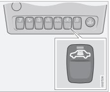
To avoid inadvertently triggering of the alarm for example when leaving a dog in the car or during a ferry crossing - the movement and tilt detectors can be temporarily switched off.
