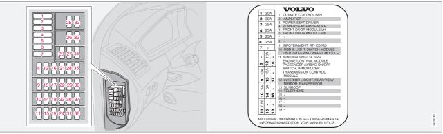
A decal which specifies the positions and amperages of the fuses is located in the end box cover.
