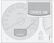
Increase or decrease the speed by pressing and holding + or –. The speed of the car when the button is released is set as the new speed.
