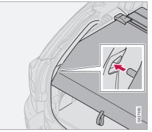
Pull out the cargo area cover, pull it over the cargo and hook it into the holes in the rear pillars of the cargo area.
