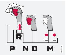
The gear selector can always be moved freely between N and D. Other positions are locked with a latch that is released with the inhibitor button on the gear selector.
