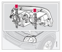
Refit the headlamp insert in reverse order. Check that the lock pins are correctly situated.
