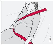
The seatbelt should always be worn during pregnancy. But it is crucial that it be worn in the correct way. The diagonal section should wrap over the shoulder then be routed between the breasts and to the side of the abdomen.
