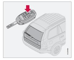
If the car is equipped with an alarm<sup>\*</sup> the alarm indicator on the instrument panel stops to show that alarm for the whole of the car is not armed. The alarm's level and movement sensors and the sensors for opening the tailgate are disconnected.
