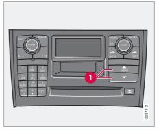
Some infotainment system functions are controlled via a menu system. The current menu level is shown at the top right of the display. Menu options are shown in the middle of the display.
