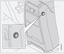
Button for rear seat heating, On/Off.
