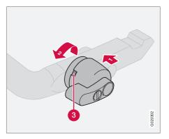
Check that the indicator window (3) shows red. If the window does not show red, press in (1) and turn the locking wheel anticlockwise (2) until you hear a click.
