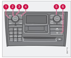
Press the **POWER** button **2** to switch the audio system on or off.
