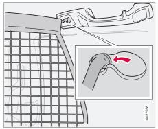
The safety net prevents luggage and cargo from being thrown forward in the passenger compartment during heavy braking.
