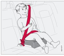
Volvo's integrated booster cushion for the centre rear seat is specially designed to provide optimum safety for children. Combined with the regular seatbelts the integrated booster cushion is approved for children weighing between 15 and 36 kg.
