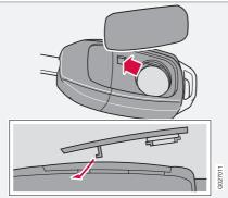
Replace the battery after repeated failure by the locks to respond when remote control key signals are transmitted within a normal distance.
