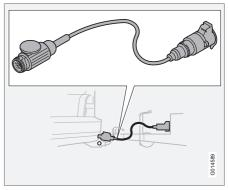
An adapter is required if the car's towing bracket has 13 pin electrics and the trailer has 7 pin electrics. Use an adapter cable approved by Volvo. Make sure the cable does not drag on the ground.
