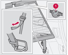
The safety net can be folded up and placed in the cargo area floor (for cars seating five).
