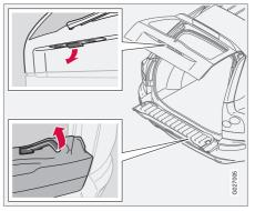
Open the tailgate by pulling the handle indicated in the illustration. Fold down the rear flap by lifting the handle up.
