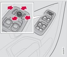
The controls for adjusting the two door mirrors are at the front of the driver's door armrest. The rearview mirrors can be operated in ignition position I and II.
