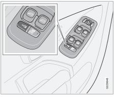
Automatic locking is activated and deactivated from the control panel in the driver's door. The function operates by locking the doors automatically when the speed of the car exceeds 7 km/h. They remain locked until a door is opened from the inside or when all doors are unlocked from the control panel.
