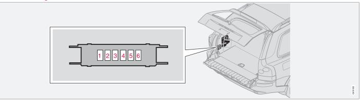
The fuse box is located behind the cover panel on the left-hand side.
