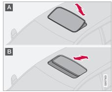
The sunroof controls are located in the roof panel. The sunroof can be opened in two positions:
