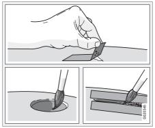
Before touching up paintwork, the car must be clean and dry and at a temperature above  $15 \, {}^{\circ}\text{C}.$
