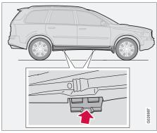
Remember to set out the warning triangle if you must change a wheel in a trafficked area. There are two jacking points on each side of the car. The jacking points are centred under the bottom of the doors.
