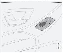
The rear door windows can be operated with the controls on the doors and the switch on the driver's door. If the light in the switch for blocking power windows in the rear doors (located in the driver's door control panel) is illuminated, the rear door windows can only be operated from the driver's door.
