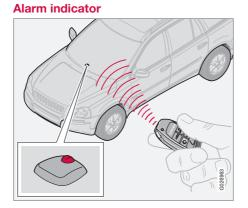
A red LED on the instrument panel indicates the alarm system's status:
