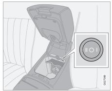
There is a cooler box under front seat's folding armrest. Adjust the cooling level with the button (see illustration). The cooler box works when the engine is running or in key position **II**.
