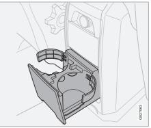
Pull the bottom edge of the insert to open.
