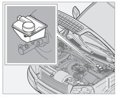
Brake and clutch fluid have a common reservoir<sup>1</sup>. The fluid level must be between the **MIN** and **MAX** marks. Check the level regularly. Change the brake fluid every other year or at every other regular service.
