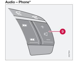
The four buttons at the bottom of the steering wheel keypad control both the radio and the phone. The function of the respective button depends on which system is active. The steering wheel keypad can be used to adjust volume, switch between preset stations and change CD tracks. The two upper buttons in the keypad (**Yes** and **No**) are used to answer and end phone calls respectively.
