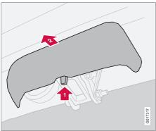
Remove the protective cover by first pressing in the catch i and then pulling the cover straight back 2.
