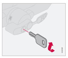
2. Ensure that the mechanism is in the unlocked position by turning the key clock-wise.
