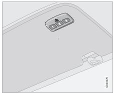
HomeLink<sup>®</sup> is a programmable remote control which can control up to three different devices (e.g. garage door, alarm system, outdoor lighting and indoor lighting etc.) and in doing so replace their remote controls. HomeLink<sup>®</sup> is supplied built into the left-hand sun visor.
