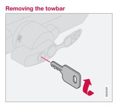
1. Insert the key and turn it clockwise to the unlocked position.
