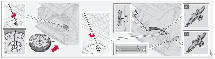
The spare wheel is located under the car. The jack\*, tool kit\* and crank are located under the floor hatch. The crank is in two parts. One part is in the tool kit, and the other is under the tool kit.
