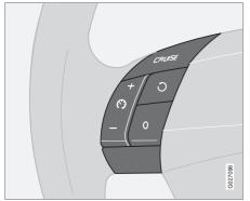
The controls for cruise control are to the left of the steering wheel.
