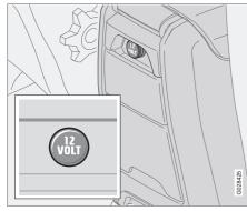
The electrical socket can be used for various accessories, such as mobile phone chargers and coolers. It is designed for 12 V. The maximum current is 10 A. For the socket to supply current, the remote control key must be in at least position **I**.
