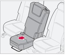
The centre seat in the second row can be slid farther forward than the other seats. Sliding the seat completely forward improves contact between a child sitting on the integrated booster cushion and front seat occupants.
