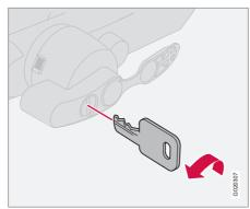
6. Turn the key anticlockwise to locked position. Remove the key from the lock.
