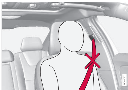
Incorrect height adjustment
