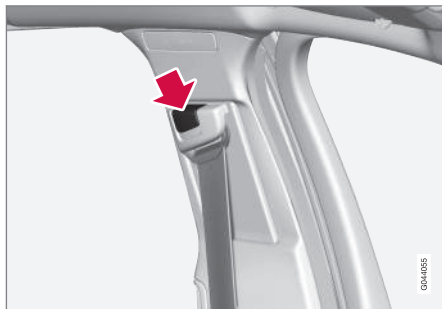
Adjusting seat belt height
