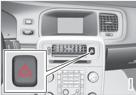
Location of the hazard warning flasher button
