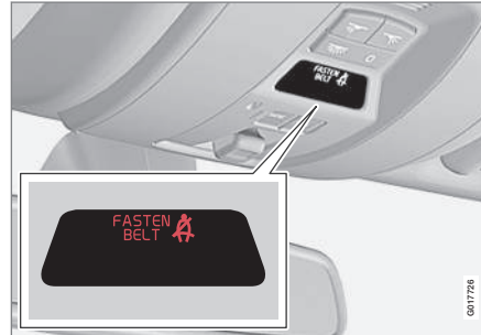
Seat belt reminder light in ceiling console
