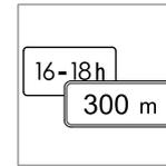
Some speed limits only apply after a certain distance or at a certain time of day. The driver's attention is drawn to this fact by means of a symbol for an additional sign below the speed symbol. The additional symbol
