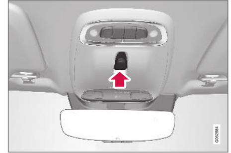
The sunroof is operated with a control located in the roof. The control is activated when the car's electrical system is in ignition position **I** or **II**.
