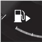
In the driver display, the arrow next to the tank symbol indicates which side of the car the fuel filler flap is located.
