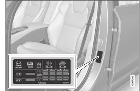
The decal displays the designation for the factory-fitted tyres on the car, as well as load limits and tyre pressure.
