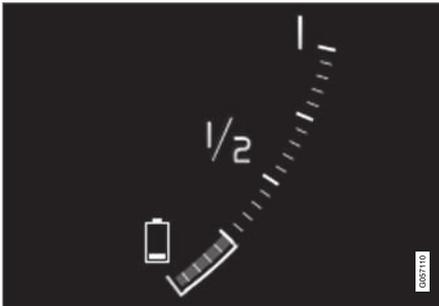
1. If the state of charge is high – run the car until approx. 25% remains. If the state of charge is low – charge the battery until a level of approx. 25% is reached.
