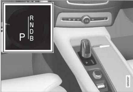
The driver display shows the gear position selected:
