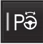
The function first checks if a space is large enough and if so then assists the driver to steer the car into the space.
