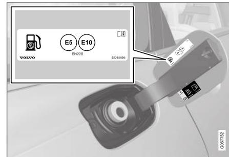
Choose fuel that is approved for use in the car in accordance with the identifier<sup>10</sup> on the inside of the fuel filler flap. See information on approved fuels and identifier in the section on "Petrol".
