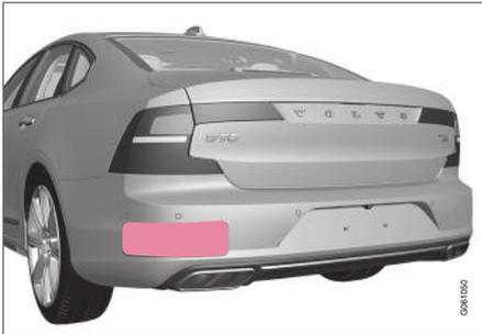
Keep the surface indicated clean – on both the left and right-hand sides of the car<sup>74</sup>.
