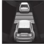
The time interval is only adjusted to the vehicle ahead by the ACC when the distance symbol shows two vehicles.
