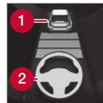
Pilot Assist steering assistance is only active when the steering wheel symbol (2) has changed from GREY to GREEN.
