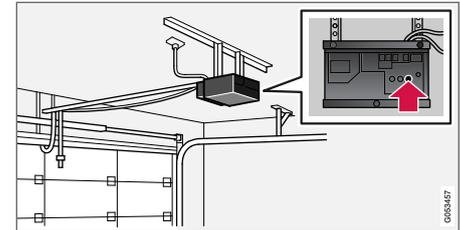
4. Locate programming button<sup>18</sup> on the receiver for the garage door or similar. It is normally located close to the antenna's bracket on the receiver.
