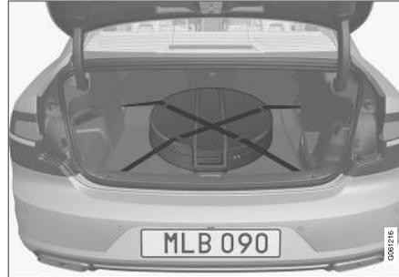
The spare wheel is stored in a bag and must be secured with two straps on the floor of the cargo area while driving. The straps must be tensioned crosswise over the wheel and attached in the car's four load retaining eyelets.
