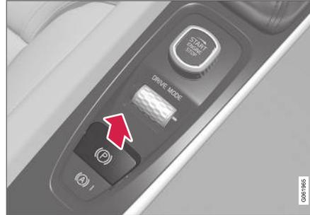
1. Pull the control upward.
