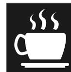
If driving behaviour becomes noticeably inconsistent, the driver is alerted by this symbol in the driver display, combined with an acoustic signal and the text message **Time to take a**
