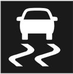
When Trailer Stability Assist (TSA) is operating, the ESC symbol flashes in the driver display.
