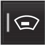
Press the **Head-up Display** button in the centre display function view. An indicator in the button illuminates when the function is activated.
