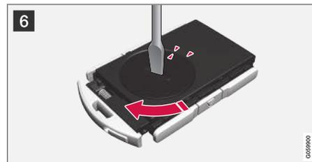
6 Refit the battery cover and turn it clockwise until the marking aligns with the **CLOSE** text.
