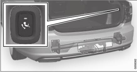
Open the boot lid. A button for extending/retracting the towbar is located on the right-hand side at the rear of the cargo area. An indicator lamp in the button must illuminate with a constant orange glow for the extension function to be active.
