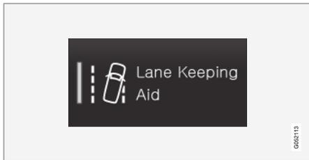
When the LED indicator illuminates in green on a function or parking button, the function is activated. When a function is activated, extra text with an explanation for certain functions is shown. The text is shown for a few seconds and then the button is shown with the LED indicator illuminated.
