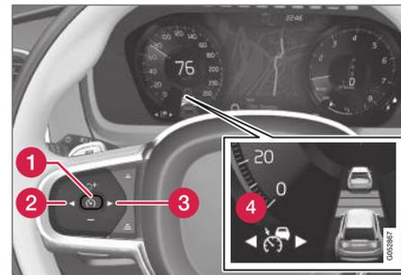
Immediately after the engine is started the Adaptive Cruise Control is in the standby mode. To set it in standby mode from active mode, proceed as follows:
