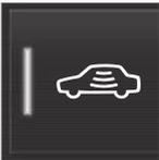
Press the **Reduced Guard** button in the centre display's function view in order to deactivate the double lock function temporarily.
