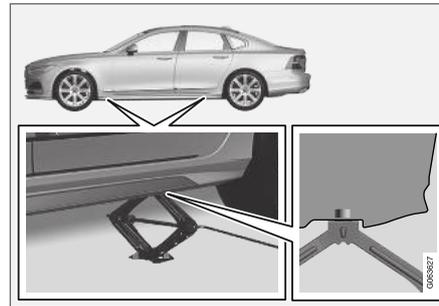
9. Position the jack on level, firm and non-slippery ground under the jacking point that will be used.
