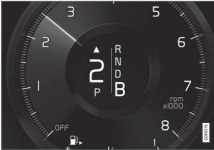
Gear shift indicator in the driver display<sup>5</sup>.
