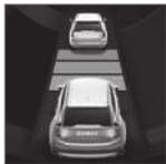
Different time intervals to the vehicle in front can be selected and shown in the driver display as 1-5 horizontal lines - the more lines the longer the time interval. One line represents about 1 second to the vehicle in front, 5 lines represents about 3 seconds.
