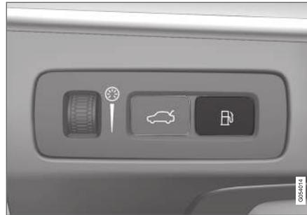
1. Press the button on the instrument panel.
