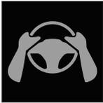
If Pilot Assist detects that the driver is not holding the steering wheel, the driver is prompted after a pause to actively steer the car, via a symbol and a text message.
