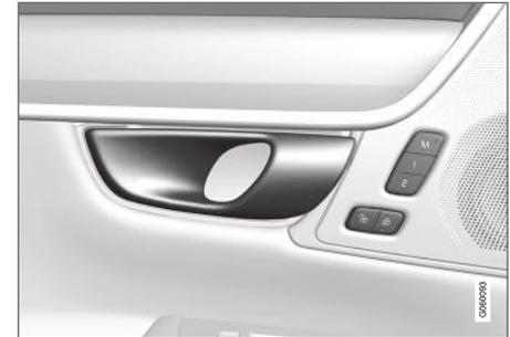
Opening handle for alternative unlocking in the side door<sup>12</sup>.
