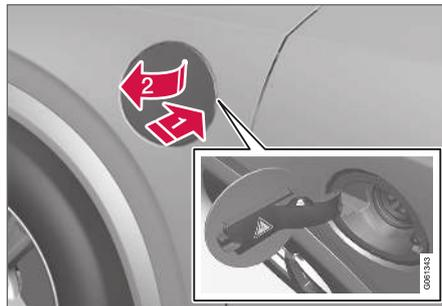
➔ Press in the rear section of the cover and release.
