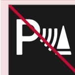
Pay additional attention while reversing when this symbol is shown if a trailer, bicycle rack or similar is mounted and electrically connected to the car.
