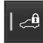
The private locking function button is located in the centre display function view. Depending on the current status of the lock, **Private Locking Unlocked** or **Private Locking Locked** is shown.
