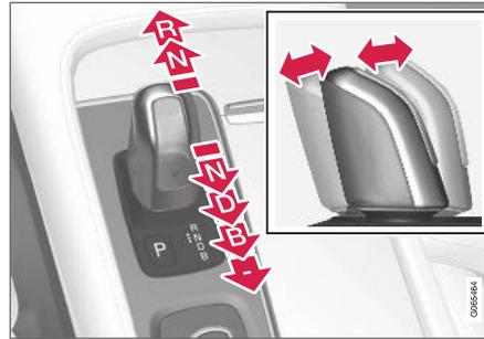
Change gear position by pressing the spring-loaded gear selector forwards or backwards.
