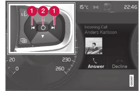
Examples of messages in the driver display and the steering wheel's right-hand keypad.
