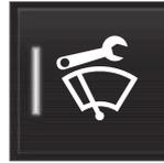
Press the **Wiper Service Position** button. The light indicator in the button illuminates when service mode is activated. When activated, the wipers move to the service position. To deactivate the service mode,
