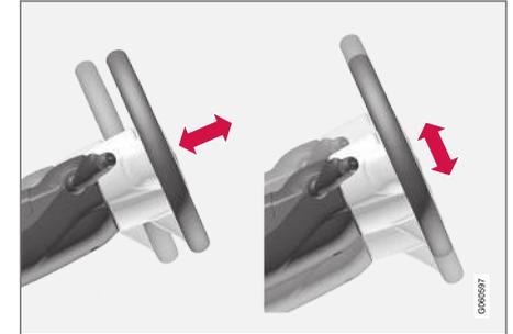
The steering wheel can be adjusted for height and for depth.
