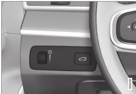
Thumbwheel (to left) for adjusting interior brightness.
