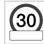
A symbol for additional sign in the form of an empty frame under the driver display's speed symbol<sup>88</sup> means that the function has detected an additional sign with supplementary information for the current speed
