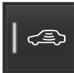
Press the **Reduced Guard** button in the centre display function view to switch off the movement and tilt sensors when subsequently locking the car.
