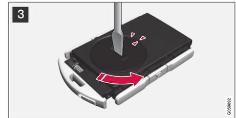
3 Use a screwdriver or similar to turn the battery cover anticlockwise until the markings meet at the **OPEN** text.
