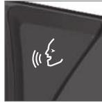
Depress the steering wheel button for voice recognition
