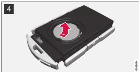
4 The battery (+) side is facing upwards. Then carefully prize loose the battery as illustrated.
