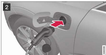
**2** Open the charging hatch. Remove the charging handle's protective cover and then press the handle the whole way into the socket for the car.
