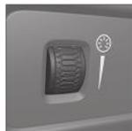
The thumbwheel on the instrument panel, to the left of the steering wheel, is used to adjust the brightness of the display light, control light, ambient light and ambience light\*
