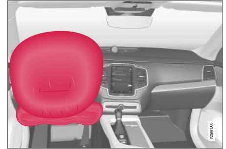
Steering wheel airbag and knee airbag on the driver's side in the front seat.
