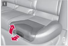
Pull the handle forward and up in order to release the booster cushion.
