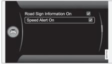
The driver can opt to receive a warning when the applicable speed limit is exceeded by 5 km/h (5 mph) or more. This warning is given by the symbol showing the applicable maximum speed temporarily flashing when this speed is exceeded. The function can be activated/deactivated in the menu system MY CAR. For a description of the menu system, see MY CAR (p. 117).
