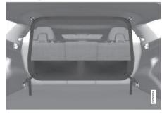
A safety net prevents loads or pets from being thrown forward in the passenger compartment in the event of sudden braking. For safety reasons, the safety net must always be correctly fastened and secured.
