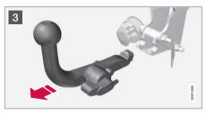
Turn the locking wheel down fully, until it comes to a stop. Hold it in this position while pulling the towbar rearward and upward.
