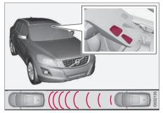
Laser sensor transmitter and receiver window12.
