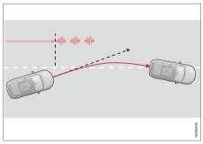
Warning with steering wheel vibration<sup>26</sup>.
