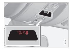
The audio reminder is speed dependent, and in some cases time dependent. The visual reminder is located in the roof console and in the combined instrument panel (p. 68).
