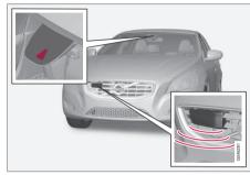
Camera and radar sensor<sup>20</sup>.
