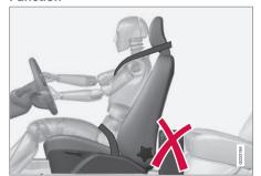
Do not leave any objects on the floor behind the driver's seat/passenger seat that may prevent the WHIPS system from functioning.
