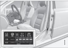
The tyre pressure label on the driver's side door pillar (between frame and rear door) shows which pressures the tyres should have at different loads and speed conditions. This is also specified in the tyre pressure table, see Tyres - approved tyre pressures (p. 439).
