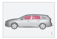
Inflatable curtain IC (Inflatable Curtain) is part of the SIPS system (p. 37) and the airbag system (p. 33). It is fitted along both sides of the headlining and helps protect the driver and passengers in the car's outer seats. A sufficiently violent collision trips the sensors and the inflatable curtain is inflated.
