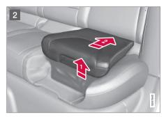
2 Lift the booster cushion up at the front edge and press it back against the backrest to lock.
