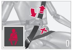
Tension the hip strap over the lap by pulling the diagonal shoulder belt up towards the shoulder. The hip strap must be positioned low down (not over the abdomen).
