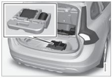
The emergency puncture repair kit is located under the floor in the cargo area.
