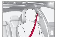
Correctly fitted seatbelt.
