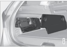
The car's tools are located behind the side hatch in the cargo area.
