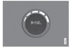
Press the switch to change between gas operation and petrol operation.
