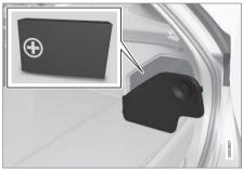
The first-aid kit is located behind the side hatch in the cargo area.
