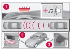
Collision warning system warning lamp and warning sound<sup>7</sup>.
