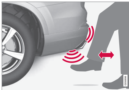
Kicking motion under the sensor's activation area
