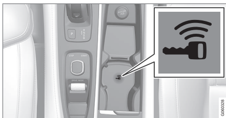
Back-up reader in the tunnel console
