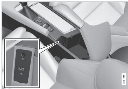
USB socket in the tunnel console
