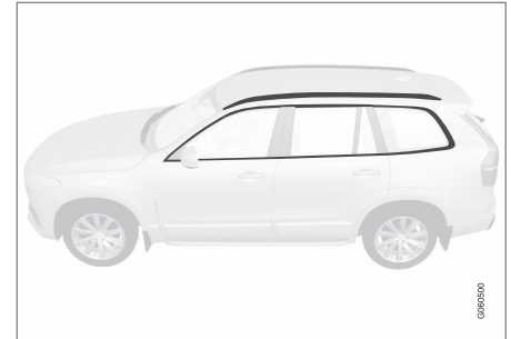
Components that should be washed with a cleaning product with a pH value between 3.5 till 11.5 (generic illustration)
