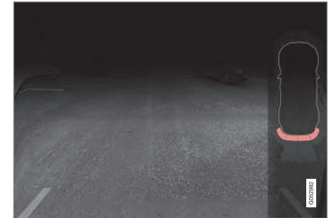
The screen can display colored sensor fields on the car symbol at the right
