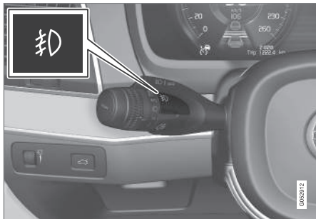
Button for front fog lamps.
