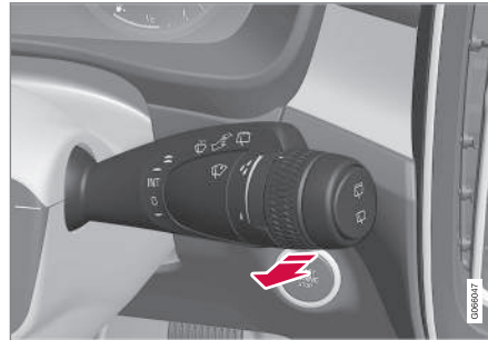
Washing function, right-hand stalk switch.
