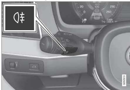
Button for rear fog lamp.
