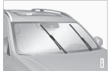
Wiper blades in service position.
