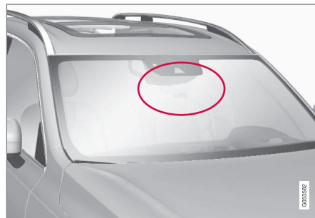
Radar unit location.
