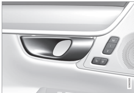
Opening handle for alternative unlocking in the side door 11 .
