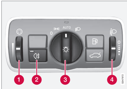
Overview, light switches.
