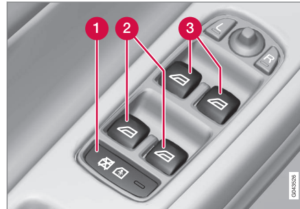
Driver's door control panel.
