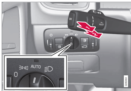
Stalk switch and knob for headlamp control.
