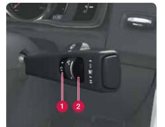
Press the lever down to start the windshield wipers or up for the single-sweep function.
