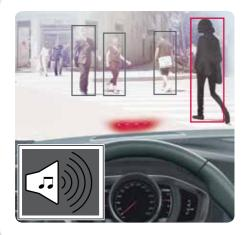
The optional Pedestrian and Cyclist Detection with Full Auto Brake system has a feature that helps detect pedestrians and applies the brakes to help slow or stop the vehicle.
