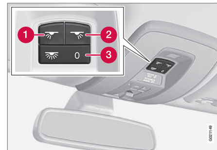
Light switches, front roof lighting
