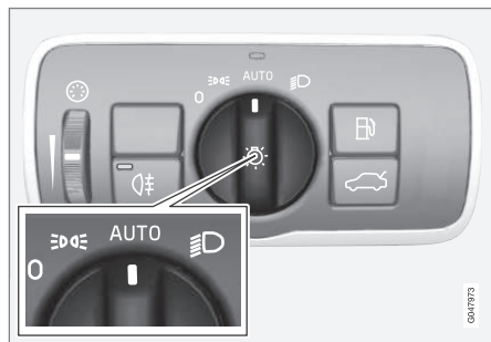
Headlight switch in the AUTO position
