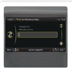
How do I connect a Bluetooth® phone? 04 Press TEL\* in the centre console. 2 Make the external device searchable/visible via Bluetooth<sup>®</sup>. 3 Press **OK/MENU** and follow the instructions on the screen. The device is now connected and can be controlled from the car. In future the phone will be connected to the car automatically.
