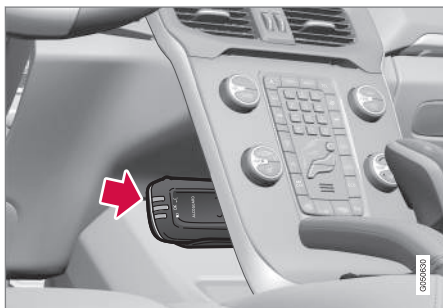
Handheld unit storage and charging station.
