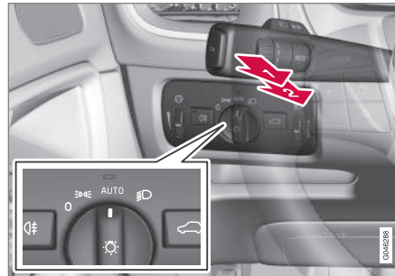
Stalk switch and knob for headlamp control.
