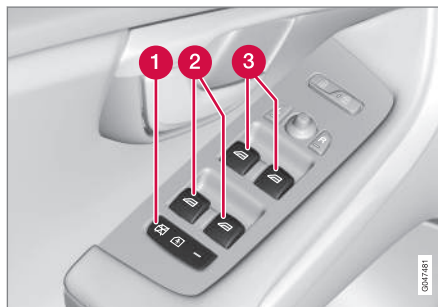
Driver's door control panel.
