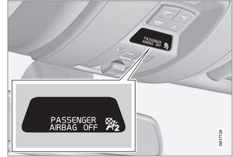
Indicator showing that the passenger airbag is deactivated.
