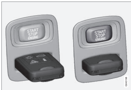
Ignition switch with remote control key extracted/inserted.
