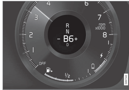
Gear shift indicator in the driver display 5 .
