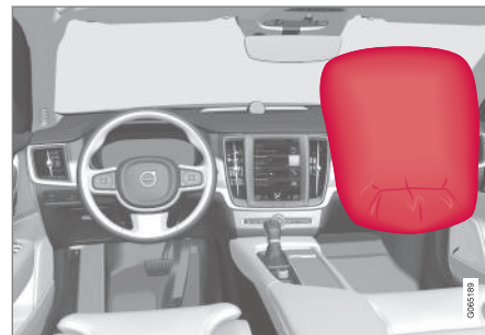
Front passenger airbag in front seat.
