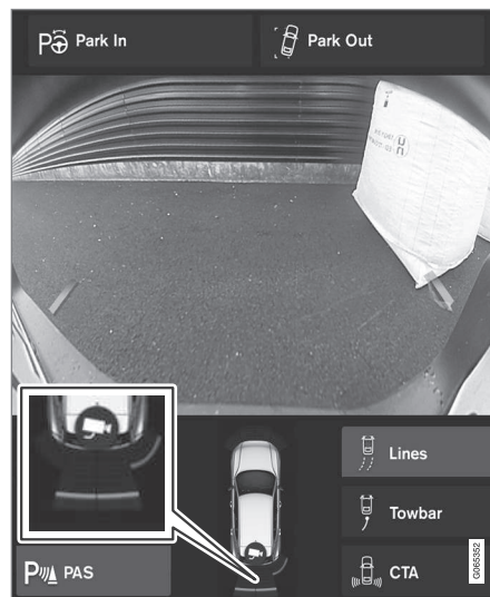
The screen can show coloured sensor fields on the car symbol.
