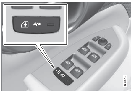
Button for electric activation and deactivation.
