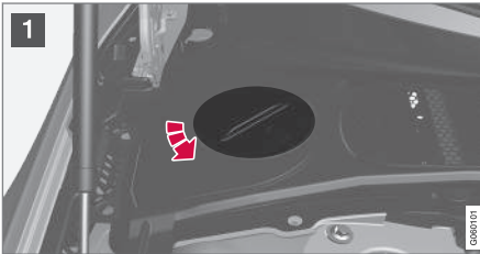
Coolant expansion tank, left-hand drive car.
