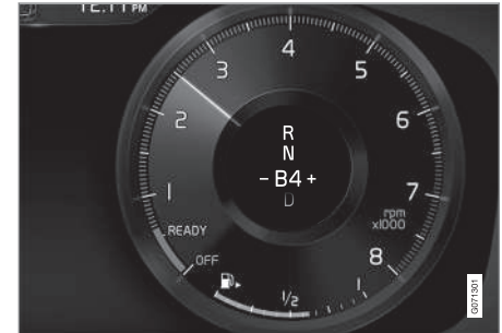
Driver display when changing gear with steering wheel paddles in manual gearshift mode.
