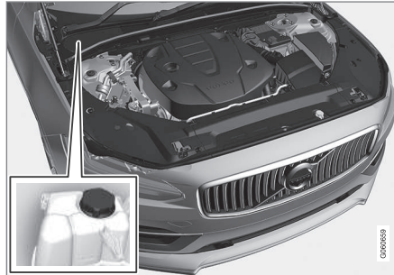
Coolant expansion tank, right-hand drive car.
