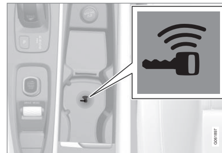
Backup reader's location in the tunnel console.
