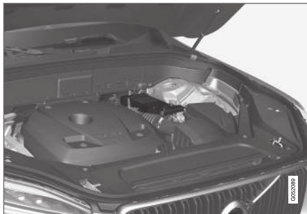
The support battery is located in a box next to the strut tower.
