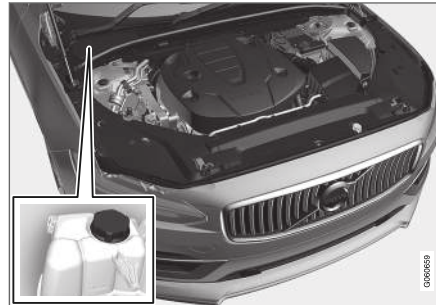
Coolant expansion tank, right-hand drive car.
