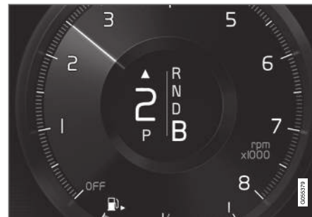
Gear shift indicator in the driver display 2 .
