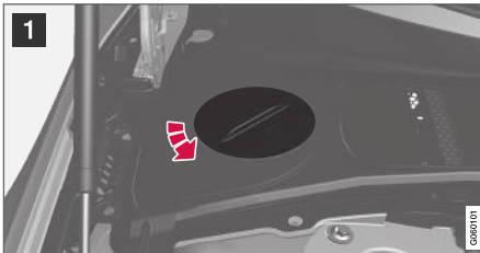
Coolant expansion tank, left-hand drive car.
