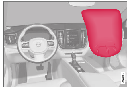
Front passenger airbag in front seat.
