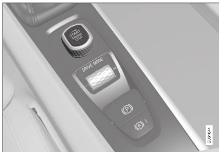
Start knob in the tunnel console.
