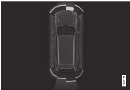
Display view showing obstacle zones and sensor sectors.
