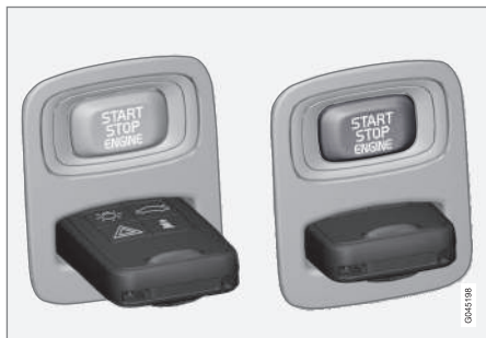
Ignition switch with remote control key extracted/inserted, and START/STOP ENGINE button.
