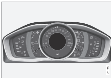
Information display, analogue instrument panel.
