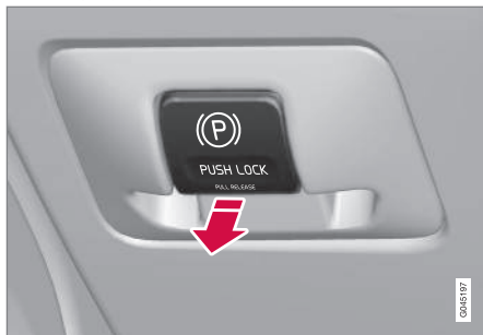
Parking brake control - release.
