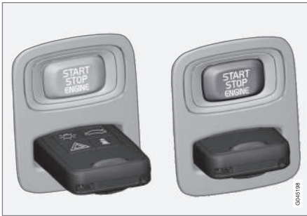
Ignition switch with remote control key extracted/inserted.
