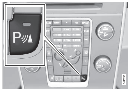
On/Off for parking assistance and CTA sensors.
