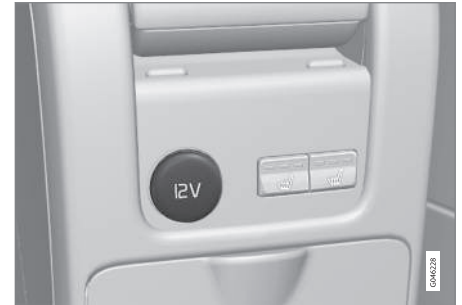
12 V socket in tunnel console, rear seat.
