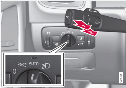
Stalk switch and knob for headlamp control.
