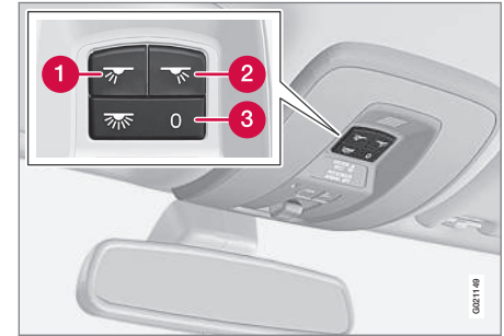
Light switches, front roof lighting
