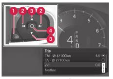
Open and navigate in the app menu<sup>2</sup> using the right-hand steering wheel keypad.
