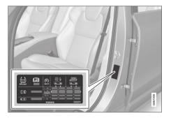
The decal specifies the designation for the factory-mounted tires on the vehicle, as well as load limits and inflation pressures.
