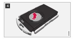
The battery's positive side (+) faces upward. Carefully pry out the battery as shown in the illustration.
