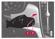
Move the right-side steering wheel lever forward to wash/wipe the rear window.
