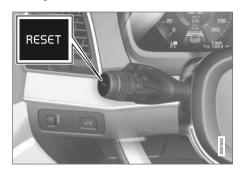
Reset all information in trip odometer TM (i.e. mileage, average fuel consumption, average speed and driving time) by pressing and holding the RESET button on the left-hand steering wheel lever.
