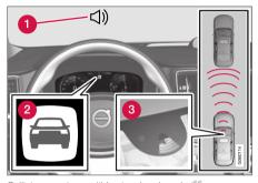
Collision warning audible signal and symbol<sup>56</sup>.
