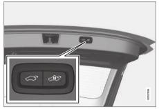
> The tailgate will close automatically - the tailgate will remain unlocked.
