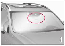
The area marked in the illustration must be kept free of decals, objects, solar film, etc.  $^{67}\,$
