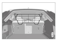
For safety reasons, the steel grid must always be installed and secured correctly.
