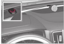
A red LED light on the dashboard will flash every other second when the vehicle is locked and the alarm is armed.
