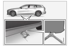
Position the jack under the attachment point being used, ensuring that the surface is firm, flat and not slippery.
