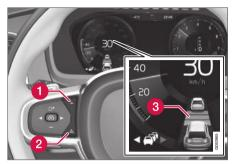
Controls for setting a time interval.
