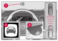
Collision warning audible signal and symbol<sup>38</sup>.
