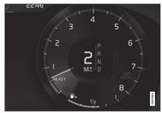
Manual shifting mode in the instrument panel<sup>2</sup>.
