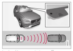
Location of the camera and radar sensor<sup>68</sup>.
