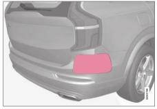
Keep the marked area clean (on both the left and right sides of the vehicle)78.
