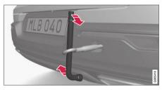
Fasten the eyelet securing by, for example, inserting a lug wrench\* through it and using this as a lever.
