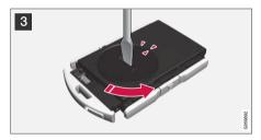
Use a screwdriver or similar object to turn the battery cover counterclockwise so the markers point to **OPEN**.
