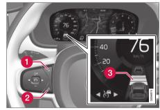
Controls for setting a time interval<sup>43</sup>.
