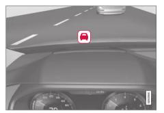
Collision warning symbol on the windshield<sup>39</sup>.
