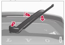
Lift the wiper arm from the window and pull the upper section of the blade down diagonally to the right.
