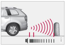
The sensors for reverse are activated if the car. rolls backward without a gear engaged or when the gear lever is moved to reverse position.
