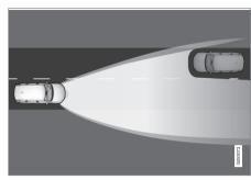
Dipped beam directly towards oncoming vehicle, but continued main beam on both sides of the vehicle.
