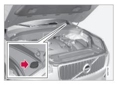
Washer fluid is filled by opening the blue cap.
