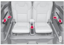
Storage compartment and cup holder in the side panel and storage space between the seats.
