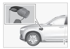
Charging cable plug and charging input socket.
