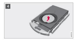
The battery (+) side is facing upwards.
