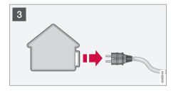
3 Unplug the cable from the 230 VAC socket. Return the charging cable to the storage space under the cargo area floor.
