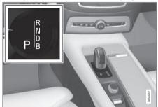
The driver display shows the gear selector's position:
