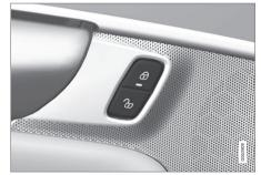
Locking/unlocking button with indicator lamp in the front door.
