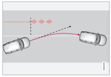
Lane assistance warns with steering wheel vibrations<sup>7</sup>.
