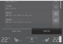
The button for editing the list/deleting the time setting in the tab **Parking climate** in the climate view.
