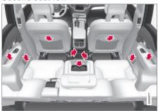
Storage compartment and ashtray\* in the door panel, cup holder\* in the centre seat backrest, storage pocket\* on the front seat backrest and also electrical sockets and cigarette lighter\* in the tunnel console.
