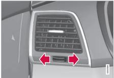
The air vent's thumbwheel<sup>1</sup>.
