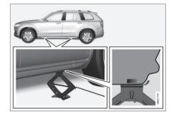
Crank up the jack so that it makes contact with the car's jacking point. Check that the head of the jack is correctly positioned in the jacking point so that the bump in the centre of the head fits into the jacking point hole and the base is positioned vertically below the jacking point. Also make sure you turn the jack so that the crank is as far away from the side of the car as possible, at which point the jack's arms are perpendicular to the direction of the car.
