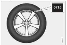
Tyres are perishable. After a few years they begin to harden at the same time as the friction capacity/characteristics gradually deteriorate. For this reason, aim to get as fresh tyres as possible when you replace them. This is especially important with regard to winter tyres. The last four digits in the sequence mean the week and year of manufacture. This is the tyre's DOT marking (Department of Transportation), and this is stated
