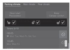
Boxes for seat heating and steering wheel heating in the **Parking climate** tab in the climate view.
