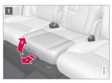
Pull the handle forward and up in order to release the booster cushion.
