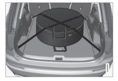
The spare wheel is stored in a bag and must be secured with two straps on the floor of the cargo area during driving. The backrests of the third row of seats must be lowered.
