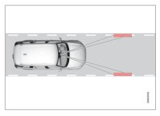
A camera detects the edge markings painted on the carriageway and compares the alignment of the road with the driver's steering wheel movements.
