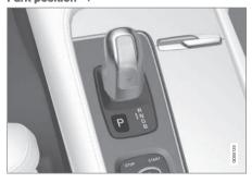
The park position is activated via the **P** button next to the gear selector.
