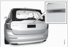
Rubber plate with pressure-sensitive surface.
