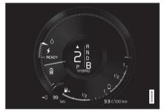
The driver display indicates charging during engine braking.
