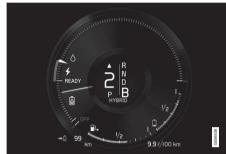
The car generates current to the battery and the battery is charged, e.g. when the brake pedal is pressed lightly or during engine braking down a hill.
