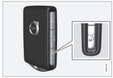
The alarm for the tailgate can be disarmed and the tailgate unlocked on its own by using the remote control key's 3 button.
