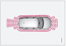
Parking assistance side sensors are activated automatically when the engine is started. They are active at speeds below 10 km/h (6 mph).
