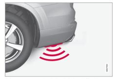
If the car is equipped with the skid plate/diffuser\* accessory, then the detector is positioned out towards the left-hand corner of the bumper.
