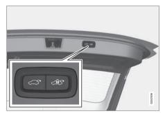
Button for closing and locking on the underside of the tailgate.
