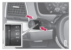
Steering wheel stalk switch with rotating ring.
