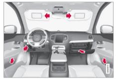
Storage compartment in the door panel and by the steering wheel, glovebox and sun visors.
