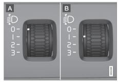
Thumbwheel positions for the different load cases.
