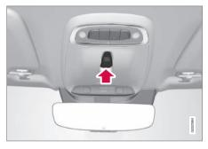
The panorama roof and curtain are operated with a control located in the roof. The control is activated when the car's electrical system is in ignition position I or II.
