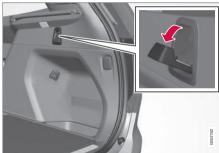
There are also two extensible bag hooks in side panels - one on each side of the cargo area.
