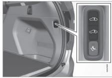
Use the buttons in the cargo area to regulate the height of the car's rear section and facilitate loading/unloading or when connecting/disconnecting a trailer. See the section "Loading".
