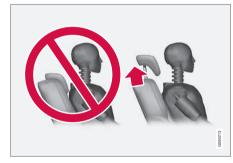
The centre seat's head restraint must be adjusted according to the passenger's height so that, if possible, the whole of the back of the head is covered. Slide it up manually as required. **4**◀
