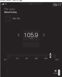
On changing over to manual tuning, the radio no longer changes frequency automatically when reception is poor.
