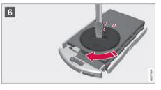
Refit the cover and turn it clockwise until the marking aligns with the **CLOSE** text.
