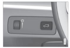
The tailgate is opened via a button on the lighting panel or on the remote control key (  $\mbox{3}$  ).
