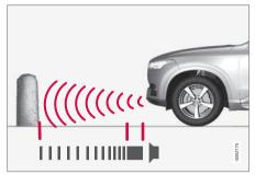
The front parking assistance sensors are activated automatically when the engine is started. The front sensors are active at speeds below 10 km/h (6 mph).
