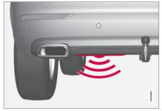
The sensor is positioned to the left of centre in the bumper<sup>17</sup>.
