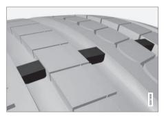
A tread wear indicator is a narrow elevation across the longitudinal grooves of the tyre's tread pattern. On the side of the tyre are the letters TWI (Tread Wear Indicator). When the tyre's tread depth is down to 1.6 mm, the tread will be level in height with the tread wear indicators. Change to new tyres as soon as possible. Remember that tyres with little tread depth provide very poor grip in rain and snow.
