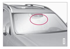
The radar unit is used by the following functions:
