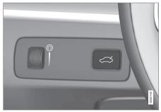
Opening/closing button on the instrument panel.
