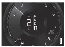
Gear shift indicator in the driver display<sup>2</sup>.
