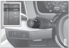
Steering wheel stalk switch with rotating ring.
