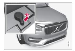
Turn the handle under the bonnet anticlockwise to release the bonnet from the lock catches and lift the bonnet.
