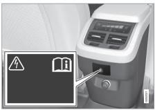
230 V electrical socket in tunnel console, second seat
