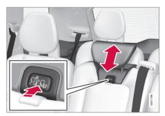
To lower the head restraint, the button (located in the centre between the backrest and head restraint, see illustration) must be pressed in while the head restraint is pressed down carefully.
