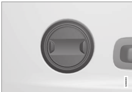
Control in cars with two-way lumbar support*.
