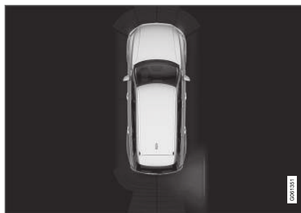
Illuminated icon for CTA in the PAS graphic on the screen 84 .
