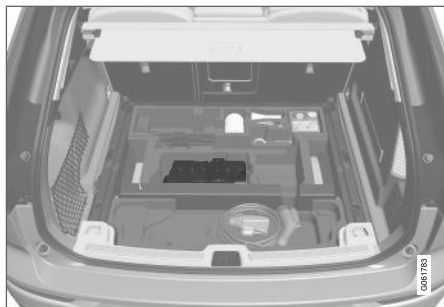
The starter battery is located in the cargo area.
