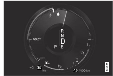
The driver display for propulsion with both the electric motor and internal combustion engine.
